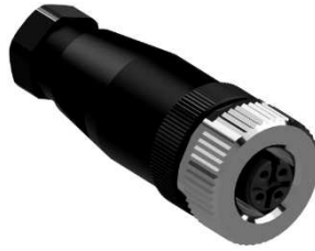
Figure 39.- Field-Wireable female connector for externally powered modules M12x1 4P, A-Code
